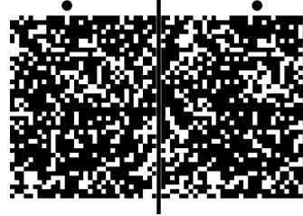
Fig. 1: An example of auto-RDS image for the perception pattern “T” shown in Fig. 2, where “•” indicates the reference point for both eyes.
