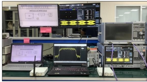
Fig. 3: Equipment for testing the QPSK communication system over the antenna.
