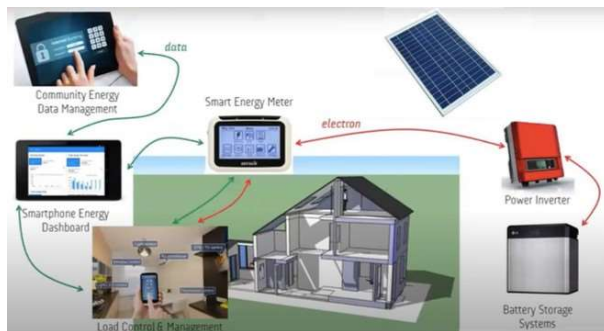
Fig.1: Smart powerwall system for energy storage system and fast charging EV
